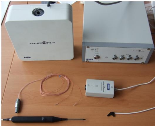
(a) Aurora components: field generator containing transmitter coils (top left), control unit (top right) and sensors coils and accessories (such as the black palate trace instrument) in the foreground (from the LORIA MAGRIT website <http://magrit.loria.fr/Confs/Issp06/>)
