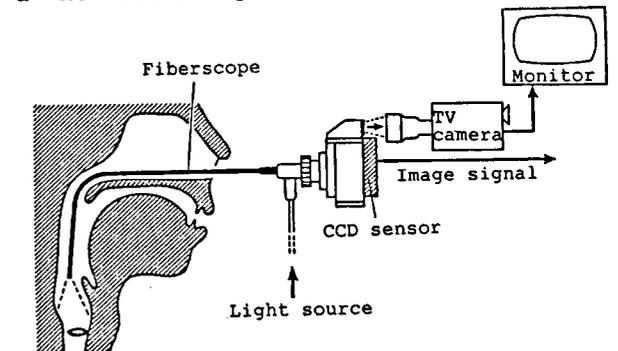
Fig. 2 Block diagram of the fiberoptic system.
