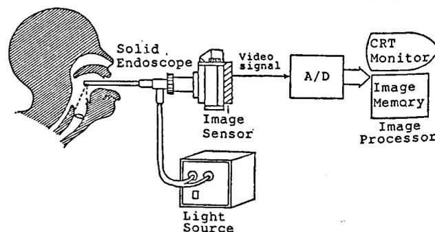
Fig. 1 Block diagram of the solid endoscope system.
