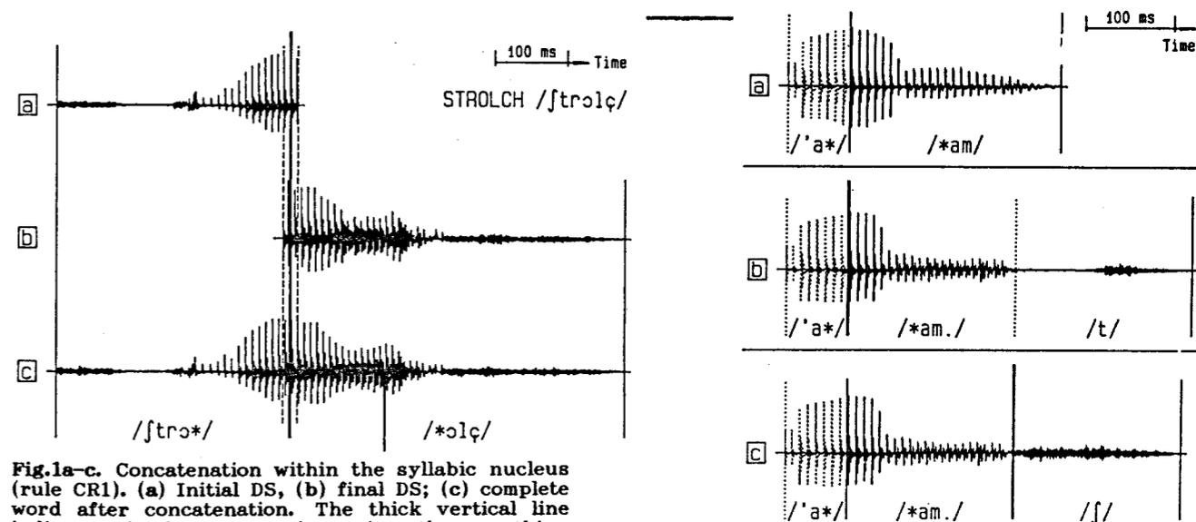
Fig.1a-c. Concatenation within the syllabic nucleus (rule CR1). (a) Initial DS, (b) final DS; (c) complete word after concatenation. The thick vertical line indicates the interconnection point; the smoothing interval is indicated by the dashed lines. The asterisk in the phonetic transcription refers to the position of the syllabic nucleus
