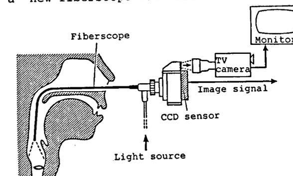
Fig. 2 Block diagram of the fiberoptic system.
