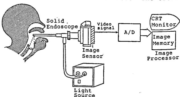
Fig. 1 Block diagram of the solid endoscope system.
