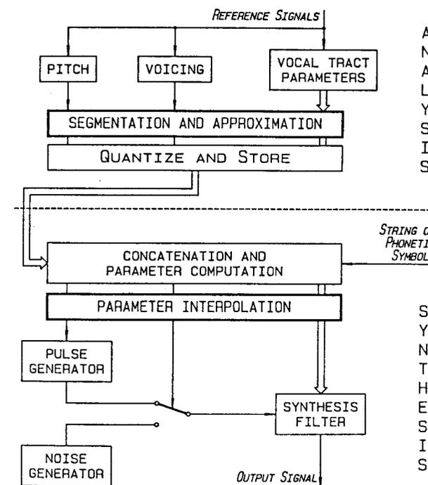
Fig.4. Vocoder configuration for speech synthesis by rule. The analysis (components above the dashed line) is done offline
