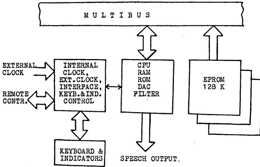
Fig. 1. The structured scheme of the compiling synthesizer.
