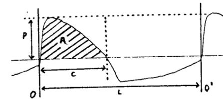
Figure 1. One period of a normal Lx waveform. Indicated are: O, O': start of closure at the onset of pitch periods; L: length (number of samples) of one period; Z: zero-line; P: maximal positive value; C: closure duration (until negative zero-crossing); A: area below the positive part of the curve.
