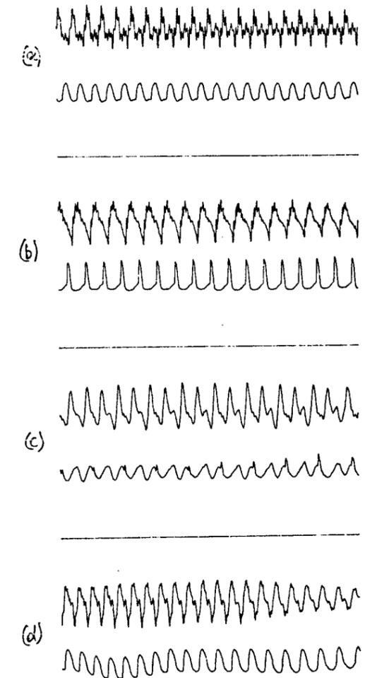
Figure 3. Sample registrations of Lx signals (lower traces) together with the acoustic speech signals (upper traces). In these examples the most noticeable deviation resides in the waveform of individual Lx periods.
