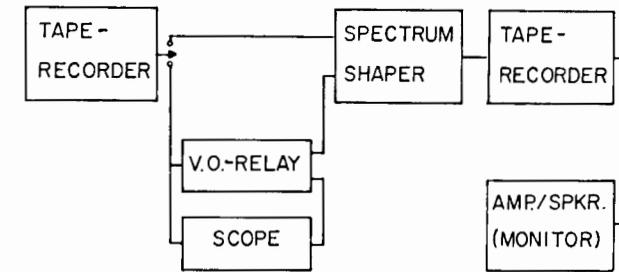
Fig. 1. Schematic of instrumentation used in modifying nasal speech of 6 cleft-palate speakers.
