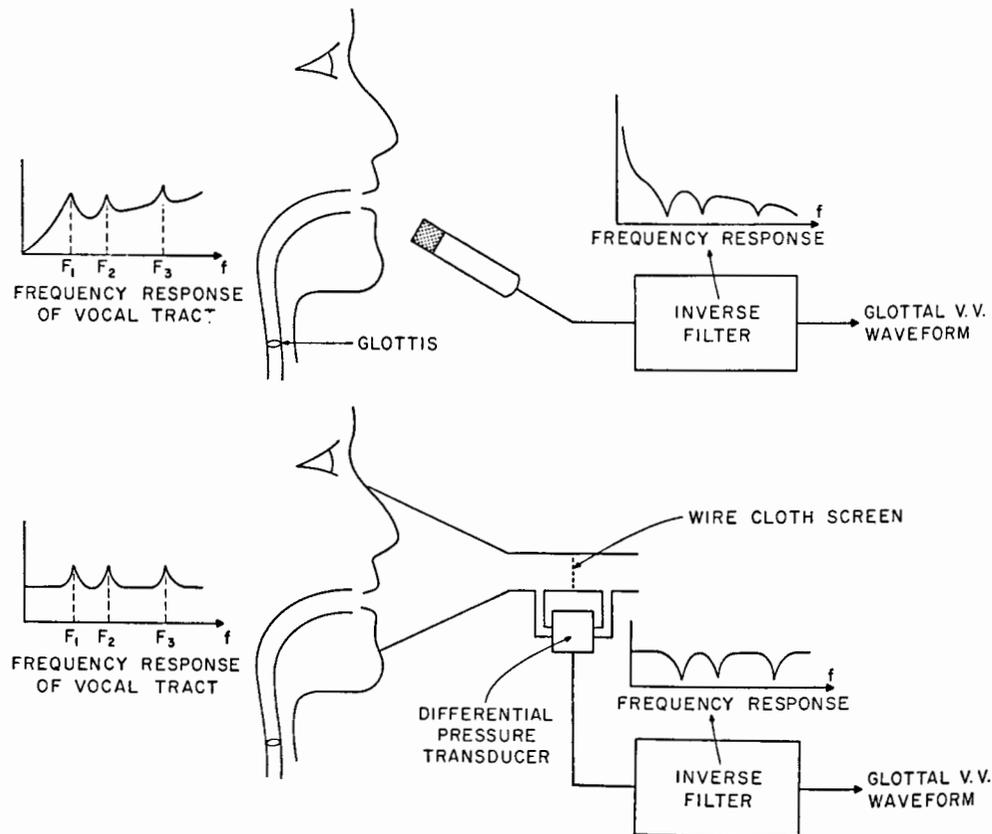
Fig. 1. Two inverse-filtering methods for obtaining the glottal volume velocity waveform: above; inverse-filtering the radiated pressure waveform, below; inverse-filtering the volume-velocity waveform at the mouth.
