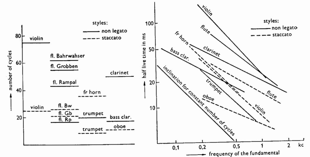
Fig. 5. Number of cycles necessary for the completion of onset for different instruments and styles.
