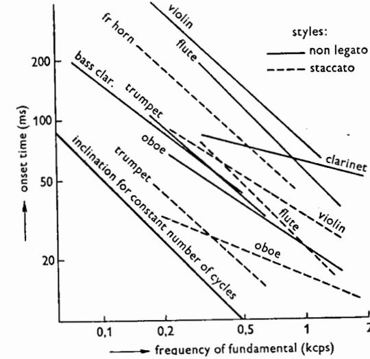
Fig. 3. Onset time as a function of frequency for different musical instruments, with the style as parameter.
