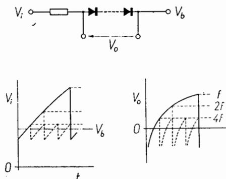
Fig. 1. Simple quasilogarithmic network transforms the initial, approximately linear, portion of an exponential function into logarithmic function within the range from  $f$  to  $4f$ .  $V_i$  — input voltage from an instantaneous frequency meter based on (3),  $V_o$  — logarithmic output fed to a differential amplifier with high input impedance,  $V_b$  — fixed bias voltage. Instead of one, several diodes are connected in series to increase  $V_b$ .
