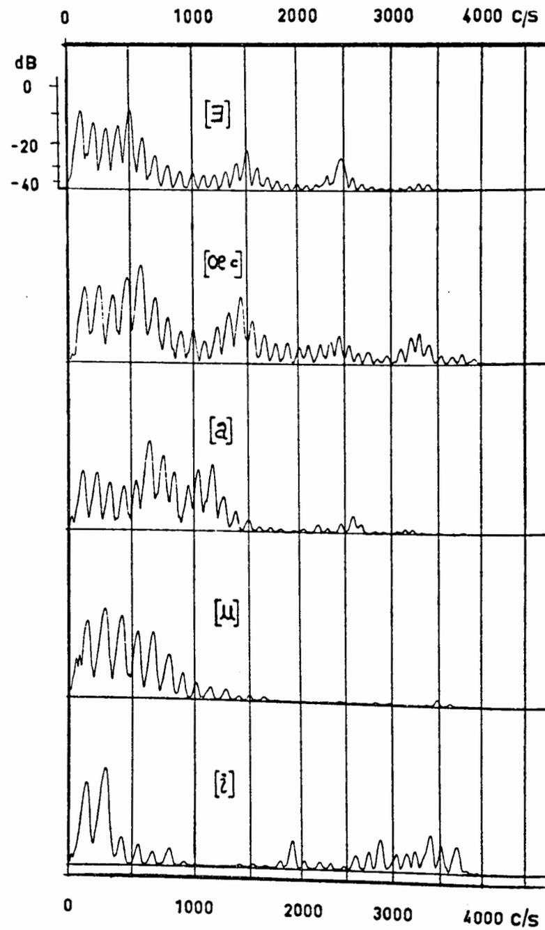
Fig. 1. Sweep frequency analysis of sustained speech sounds. The sign [ɛ] denotes a neutral reference vowel produced from OVE I. The 4000 c/s range has been run through in 3 seconds with a 31 c/s-wide filter. Mingograph recorder.
